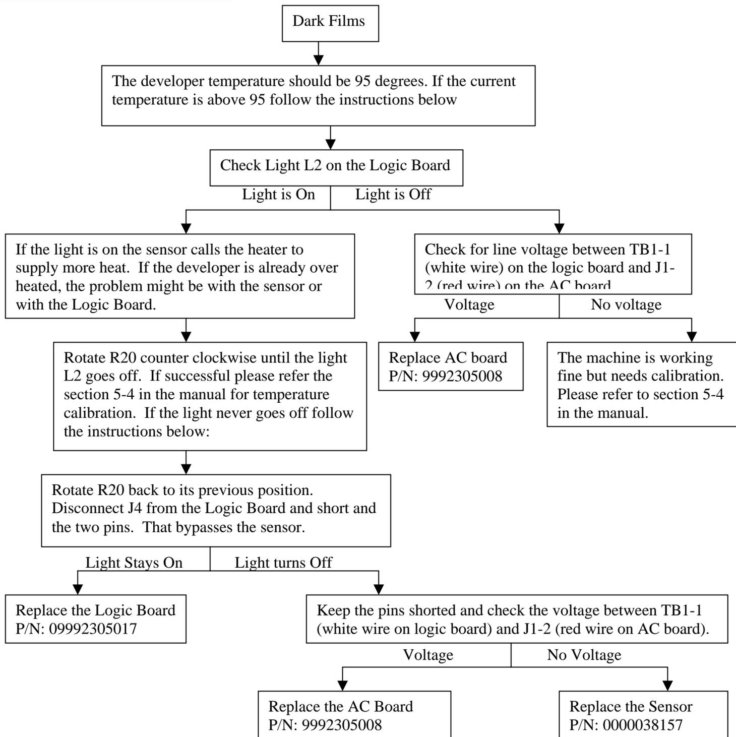
**Note: Be sure the darkroom does not have light leaks that will pre-expose the film.**
