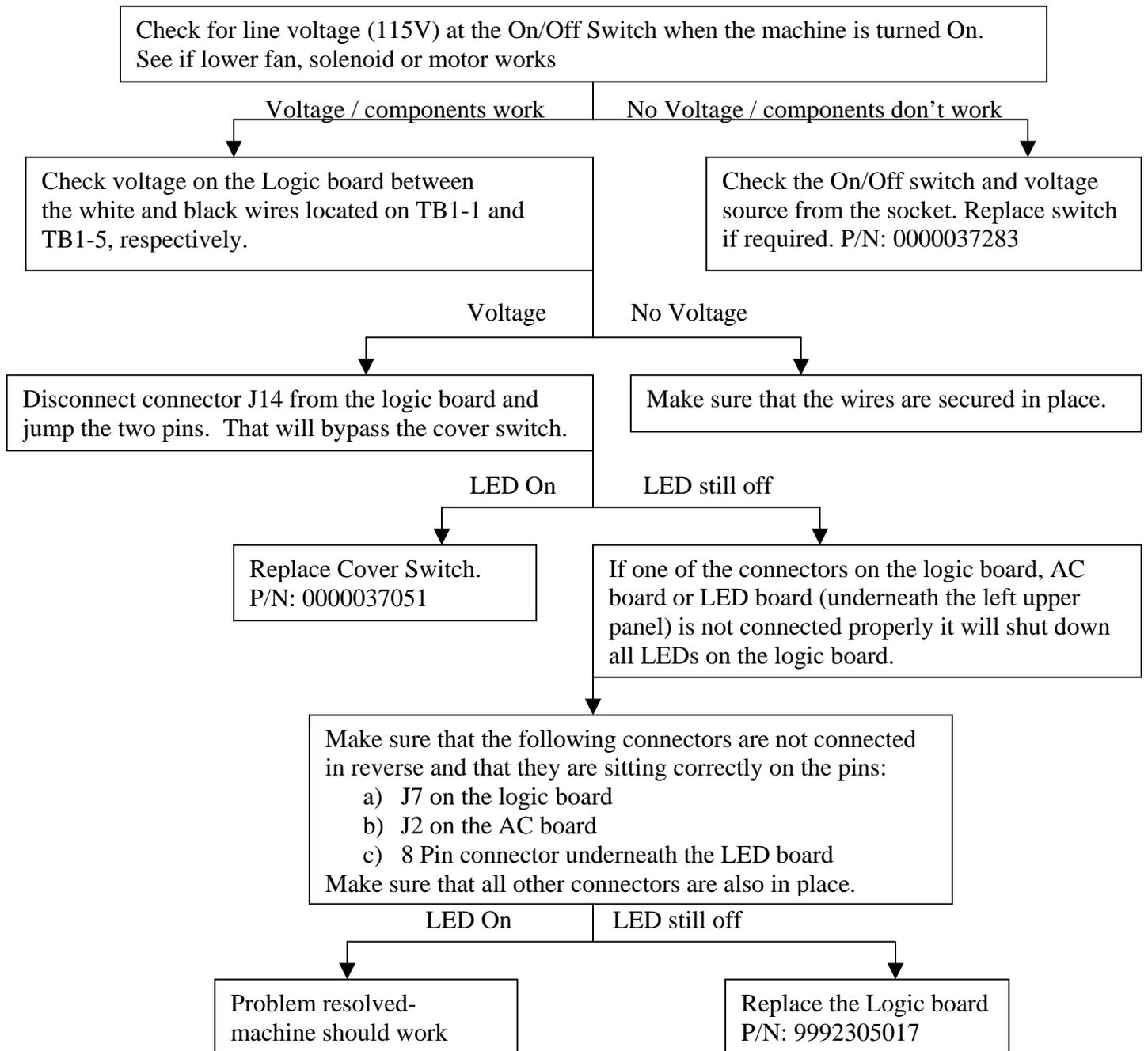
11. **The Main Breaker turns off When the Machine is turned On.**
