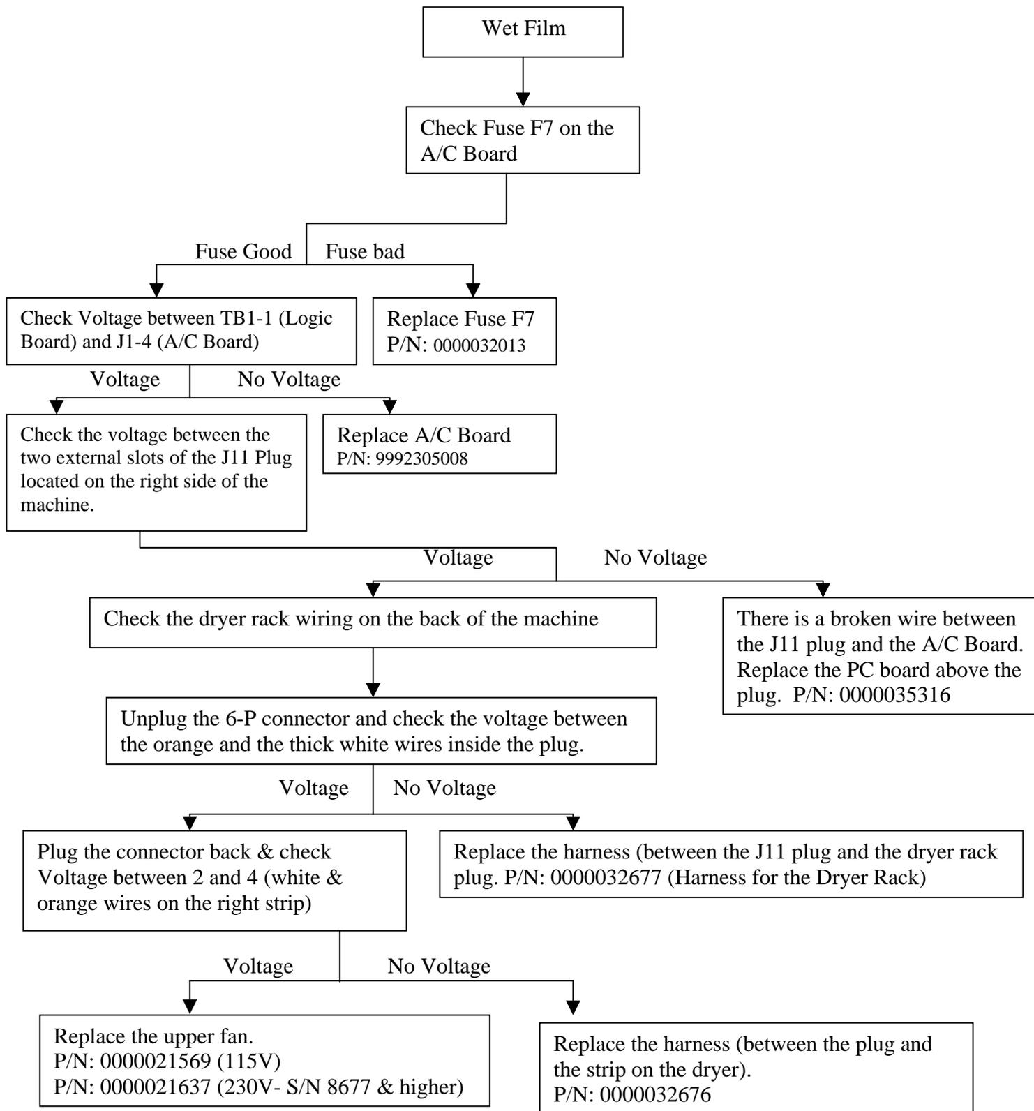
Note: If the dryer is working check / fix replenishment rates:
